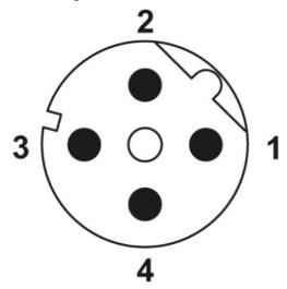
Pin assignment M12 male connector, 4-pos., male side
